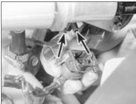
8.14b Throttle position sensor wiring plug
