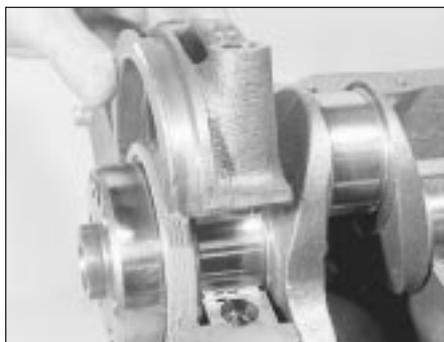
22.7 Removing the rear main bearing cap
