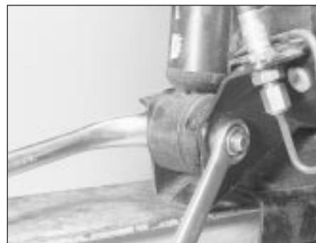
31.5 Undoing a rear shock absorber lower mounting
