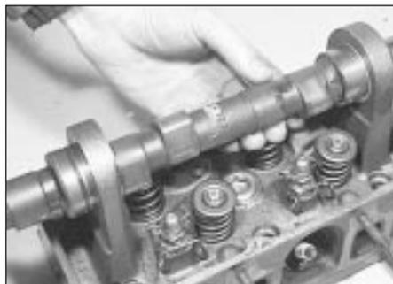
**11.8 Removing the camshaft**
