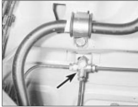
**21.7 Brake pipe union T-piece (arrowed)**
