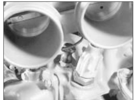
8.18a Coolant temperature sensor location
