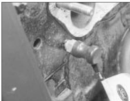
15.1a Temperature gauge sender (manifold removed)
