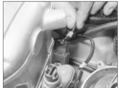
**36.47 Disconnecting a fuel injector wiring connector**
