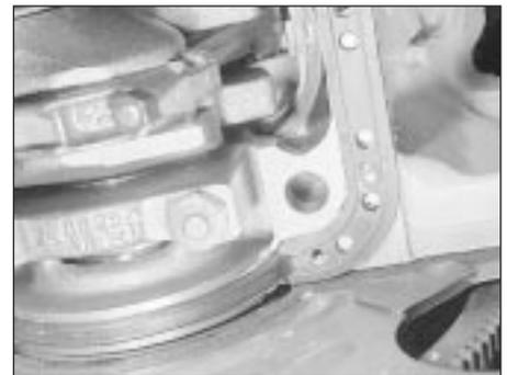
**36.28 Sump gasket at rear main bearing cap**
