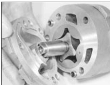
**27.3 Removing the oil pump cover**
