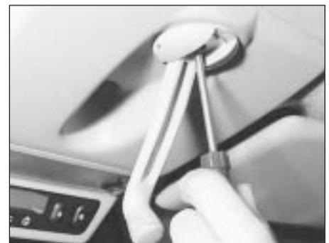
10.4 Removing the sliding roof operating handle
