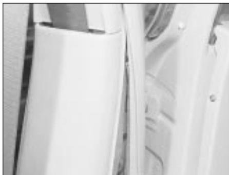
47.3 Removing the weatherstrip from the B-pillar
