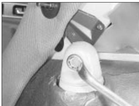
31.4 Undoing a rear shock absorber top mounting
