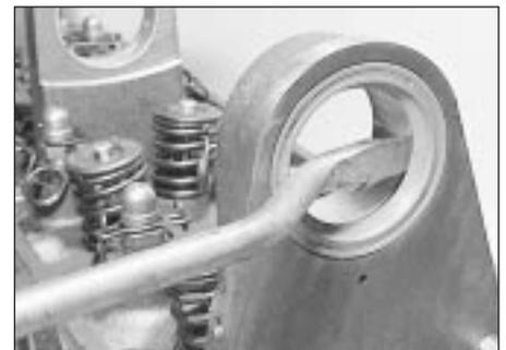
**11.9 Prise out the camshaft bearing oil seal**
