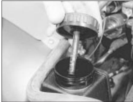
35.2 Removing the power steering fluid dipstick
