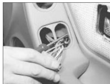
22.4b Access to the screw is through the window switch aperture
