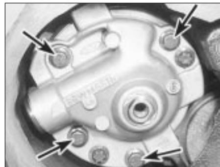
**26.3 Oil pump securing bolts (arrowed)**
