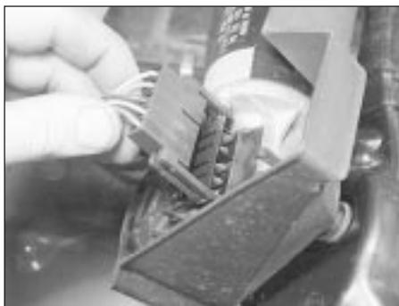
23.3 Disconnecting the wiper motor multi-plug
