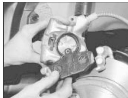
8.5 Removing a rear brake pad
