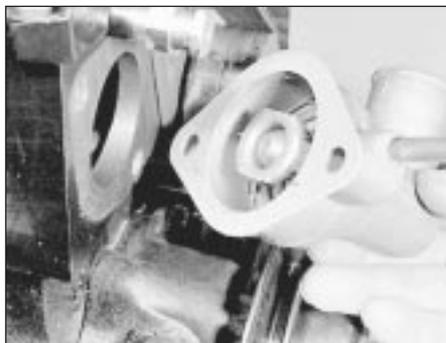
7.4 Removing the thermostat housing
