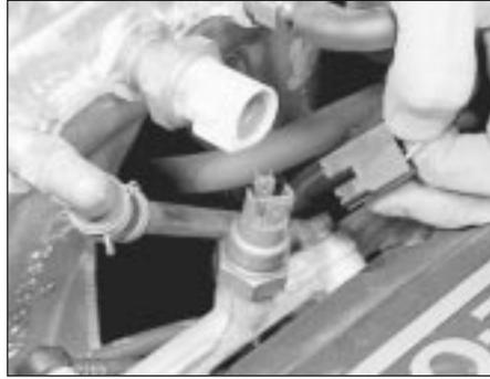
26.3 Disconnecting the fuel temperature sensor wiring plug
