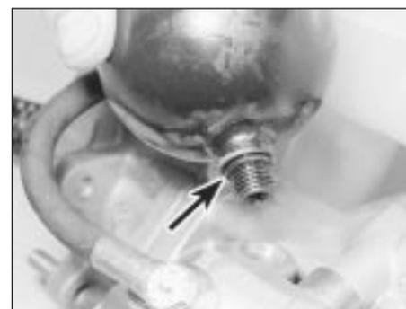
17.4 Removing the accumulator
