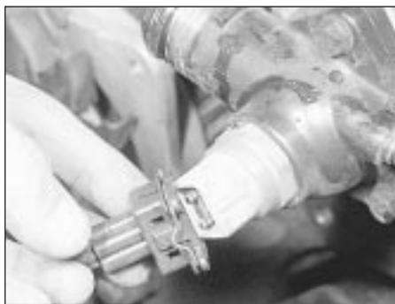
7.13 Disconnect the cooling fan switch wiring plug . . .
