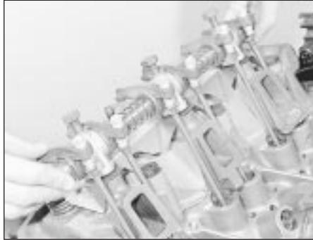
38.7b Fitting an assembled rocker shaft
