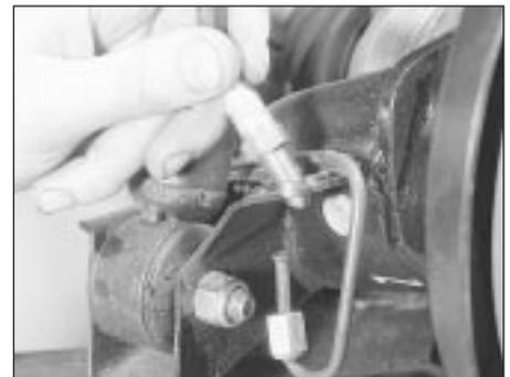
21.4 Removing a flexible hose from its bracket
