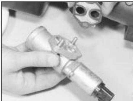
34.12 Withdrawing the idle speed control valve
