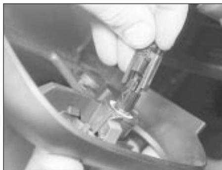
6.22 Removing the switch symbol illumination light
