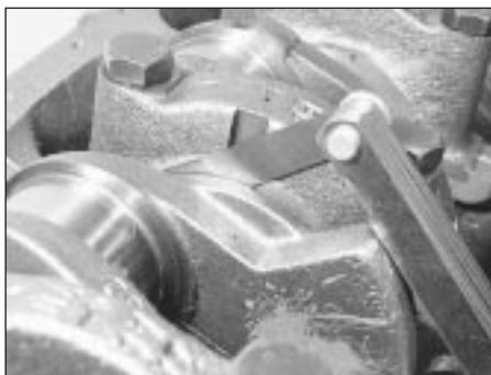
22.6 Checking crankshaft endfloat
