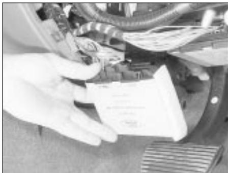
**36.6 Removing the anti-theft alarm control module**
