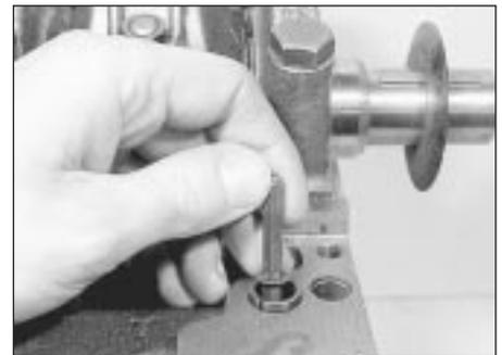
19.4 Removing the oil pump driveshaft
