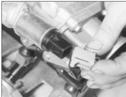
34.2 Disconnecting the idle speed control valve
