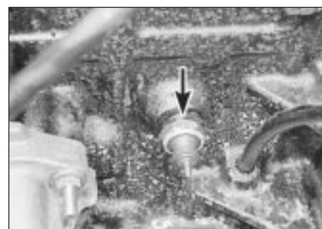
9.1a Engine oil pressure switch (arrowed)
