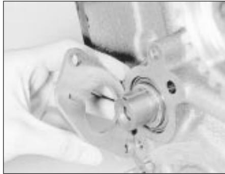
32.3b Fitting the camshaft thrust plate
