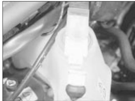
15.3b Disconnecting a fluid level sensor plug
