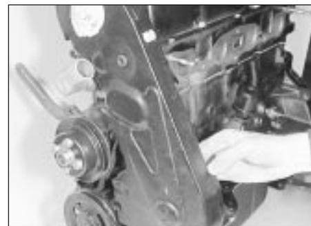
10.2 Removing the timing cover
