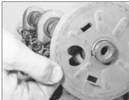
43.7 Fitting the camshaft sprocket backplate
