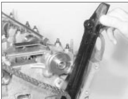
15.11c Withdrawing the lower timing chain guide
