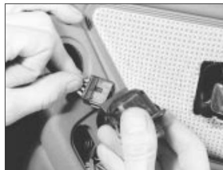
**15.15** Removing a mirror control switch
