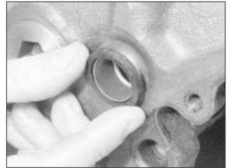
32.4 Timing cover dowel and seal
