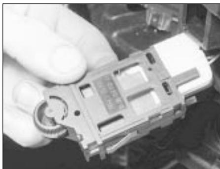
**15.10** Removing the instrument illumination dimmer switch
