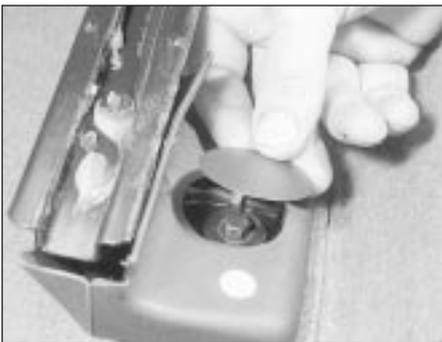
44.4a Front seat outboard rear retaining bolt
