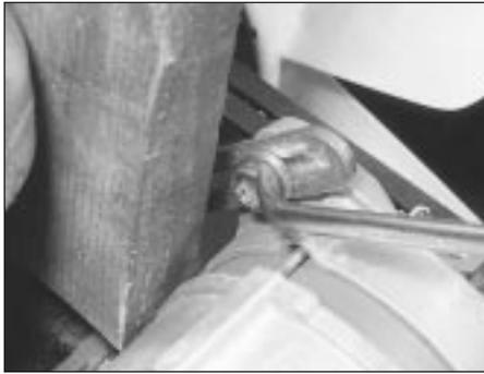
21.8 Tightening the alternator strap bolt
