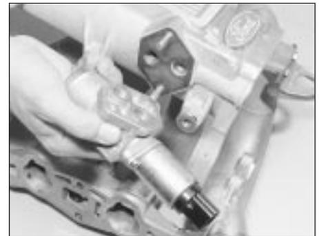
34.3 Removing the idle speed control valve
