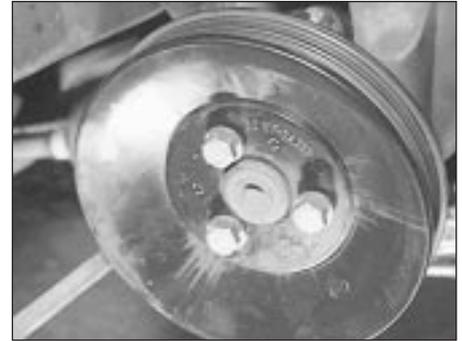
11.10 Unbolt the power steering pump pulley . . .
