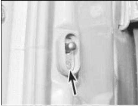
15.24 Door pillar switch securing screws (arrowed)
