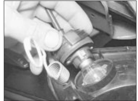
**3.20 Removing the bulb and holder from the direction indicator light unit**
