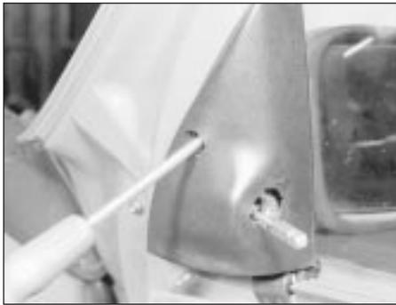
39.1a Removing the mirror mounting trim screw
