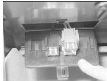
16.3 Auxiliary fuse box in the glovebox
