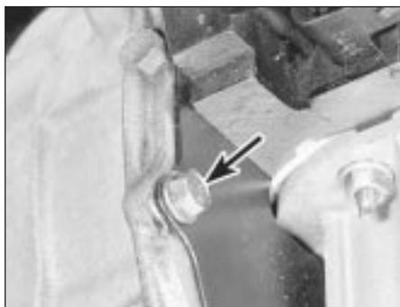
5.33 Engine adaptor plate bolt (arrowed)
