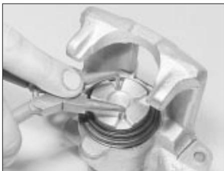
8.7 Rotating the caliper piston to retract it
