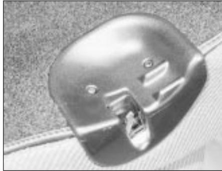
49.6 Backrest catch cover, showing securing screws
