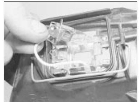
3.10 Removing the auxiliary driving light bulb
