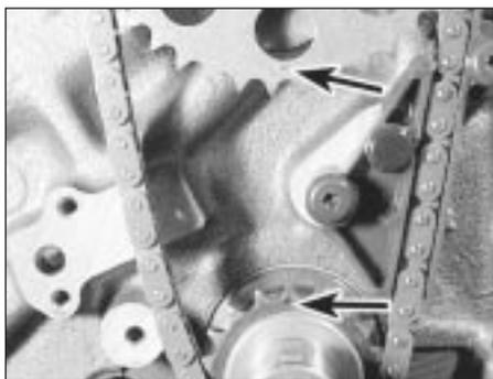
10.37 Timing sprocket alignment marks (arrowed)
