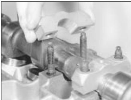
18.14a Lifting off a camshaft bearing cap
