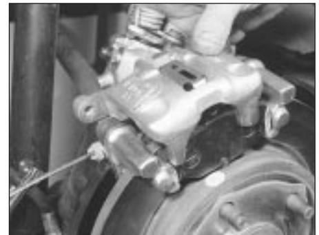
11.5b . . . and remove the rear caliper
