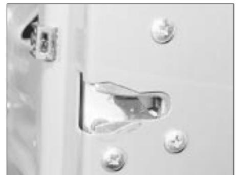
15.6 Door latch securing screws
