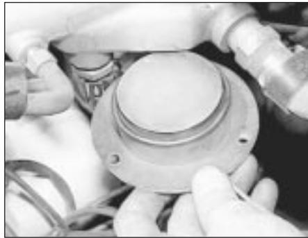
21.5 Removing the manifold heater
