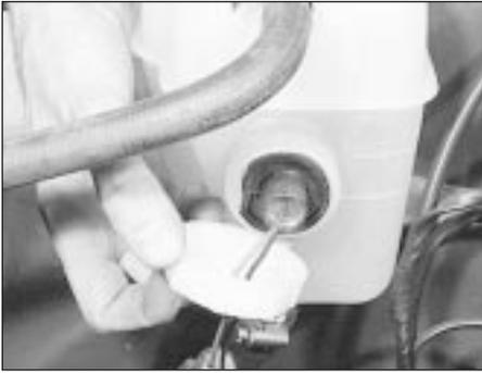
27.16 Removing the coolant level switch
