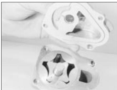
27.16b Removing the oil pump cover
