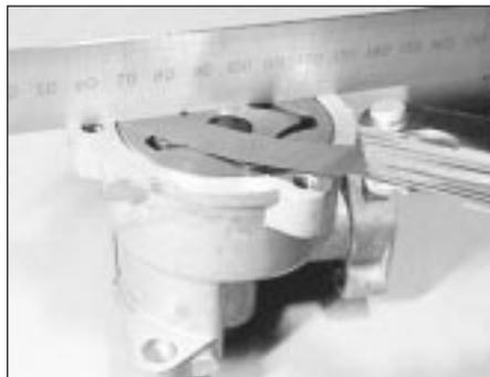
26.2c Checking the oil pump rotor endfloat
