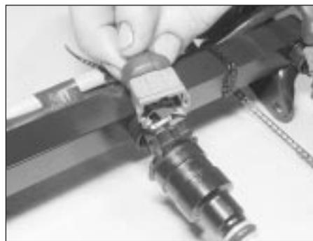
36.11 Disconnecting a fuel injector multi-plug
