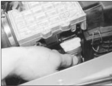
8.14a Front airflow sensor wiring plug
