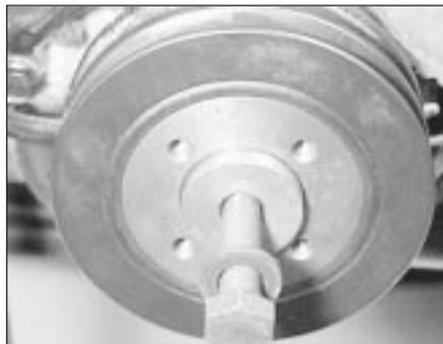
45.5b Crankshaft pulley bolt and washer
