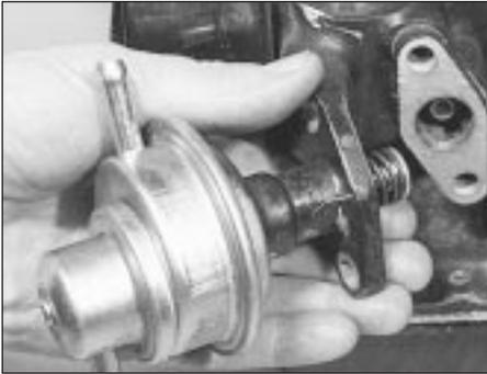
4.6a Removing the mechanical fuel pump
