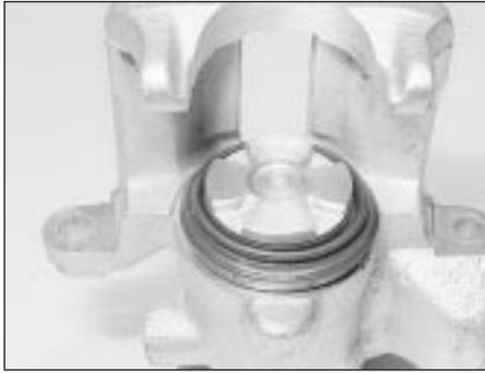
12.21 Dust boot fitted to caliper and piston
