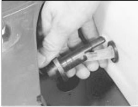
27.19 Removing the washer fluid level switch
