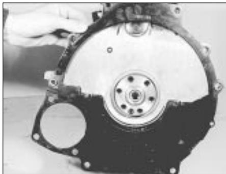
15.4 Removing the engine adaptor plate (backplate)
