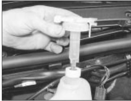
3.14 Removing the brake fluid reservoir cap
