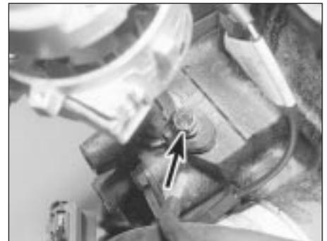
13.6 Distributor clamp bolt (arrowed)
