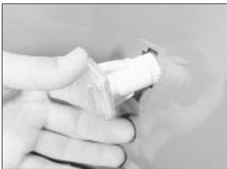
**3.24a Removing a direction indicator side repeater**
