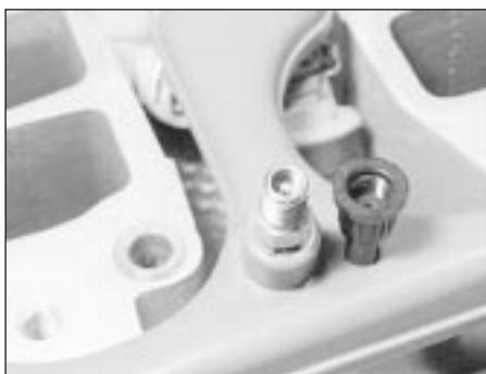
8.20 Fuel rail vent (depressurising) valve and cap
