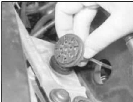
**36.9 Removing the alarm system warning buzzer**
