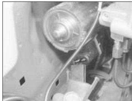
15.3e Disconnecting the pump motor plug
