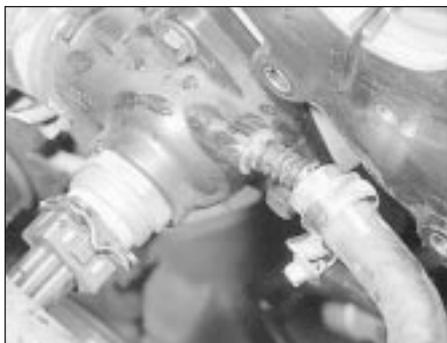
7.12a Disconnecting the coolant hoses . . .
