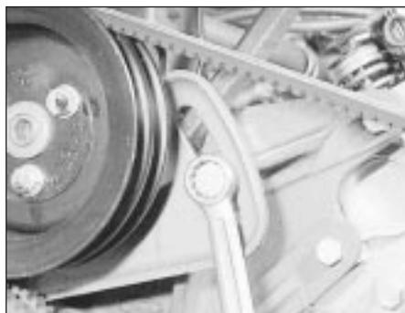
36.39b Power steering pump drivebelt tensioner bolt
