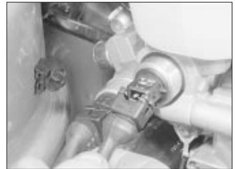
15.3c Disconnecting the main valve plug
