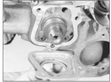
14.4 Removing the auxiliary shaft front cover
