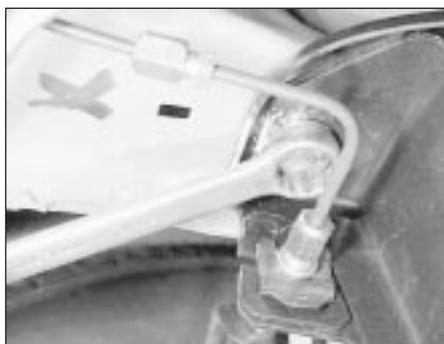
10.35 Unscrewing crossmember side bracket mounting bolts
