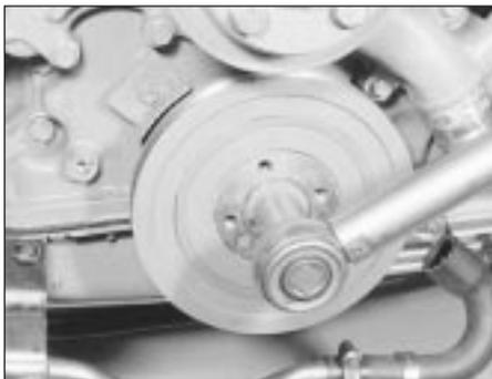
10.27a Unscrewing the vibration damper centre bolt
