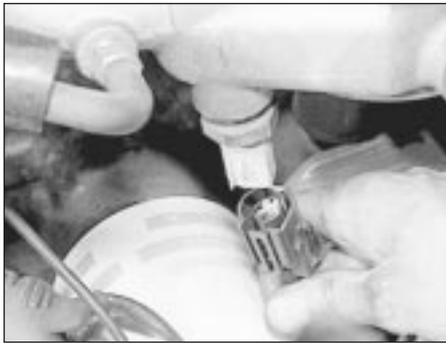
20.4 Coolant temperature sensor multi-plug
