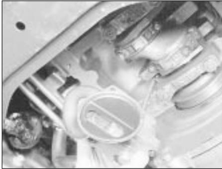
12.6 Removing the oil pump and driveshaft
