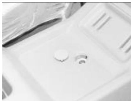
42.3 The central console securing screw (low series)
