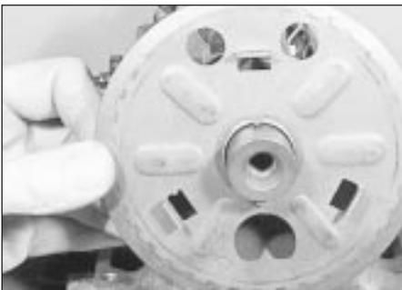
**11.3 Removing the camshaft sprocket backplate**
