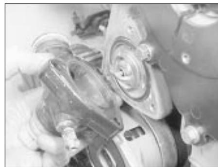
7.14 . . . and remove the thermostat housing
