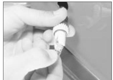
**3.24b Fitting a new side repeater bulb**
