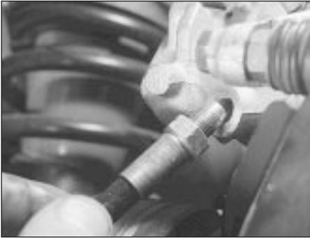
**21.5 Disconnecting the hose from the caliper**
