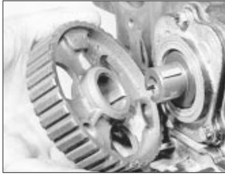
13.11 Removing the auxiliary shaft sprocket
