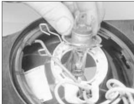
3.3 Removing a headlight bulb
