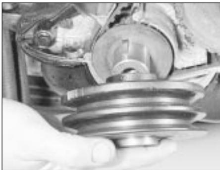
45.5a Refitting the crankshaft pulley
