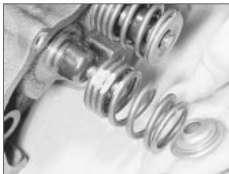
23.2b Removing the spring retainer and spring
