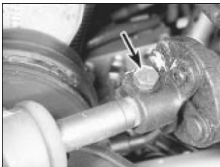
5.29 Intermediate shaft lower clamp bolt (arrowed)
