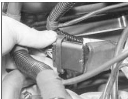
8.19a Disconnecting the distributor wiring plug
