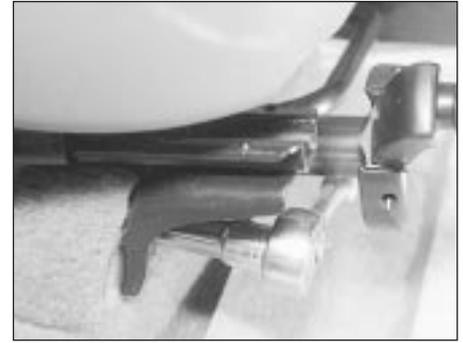
44.1 Removing a front seat retaining bolt
