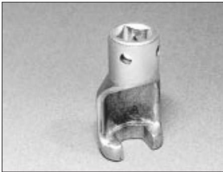
23.11 Cutaway socket spanner
