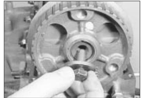
**11.2 Removing the camshaft sprocket bolt and sprocket**
