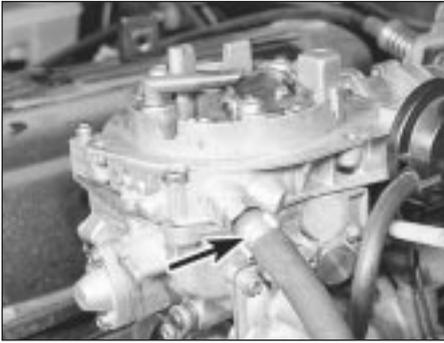
12.5 Crimped hose clip (arrowed) must be renewed
