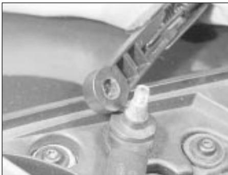
22.3b Pull the arm off the spindle
