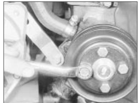
11.4 Undoing a water pump pulley bolt
