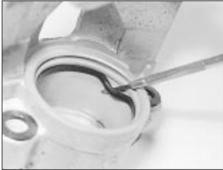
10.5 Removing the piston seal
