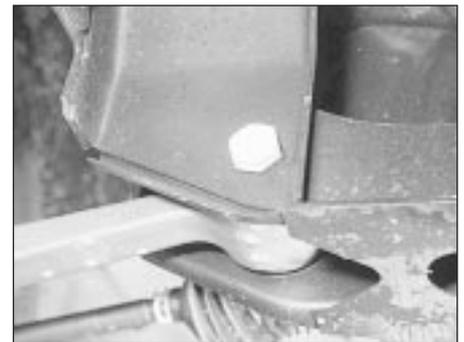
15.3 Front suspension lower arm pivot bolt
