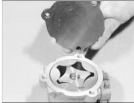
26.1 Removing the oil pump cover
