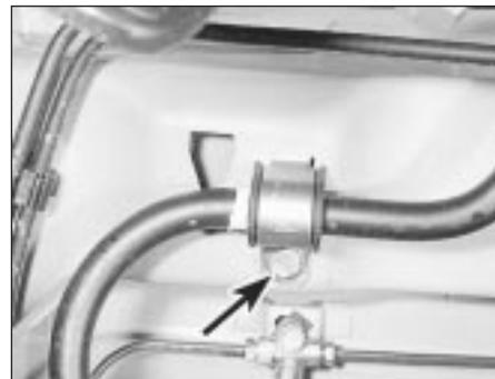
30.3 A rear anti-roll bar bracket - bolt arrowed
