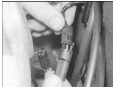
40.30 Fuel-injection wiring harness plugs
