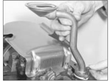
29.2 Removing the oil pick-up pipe
