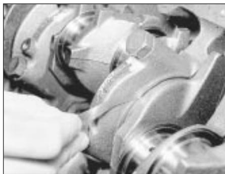
31.13 Checking crankshaft endfloat
