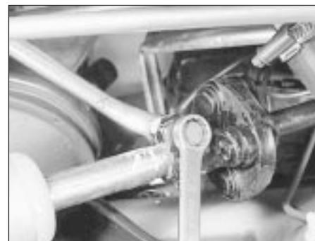
10.32 Steering shaft coupling pinch bolt
