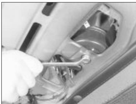
31.8 Removing a rear speaker retaining bolt
