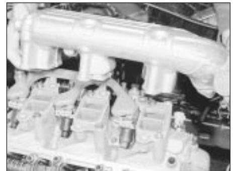
38.22 Lowering the plenum chamber into position
