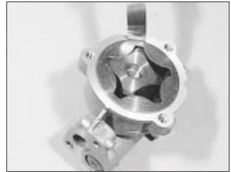
26.2a Checking the outer rotor-to-housing clearance
