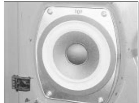
31.4 Front door loudspeaker - note TOP marking
