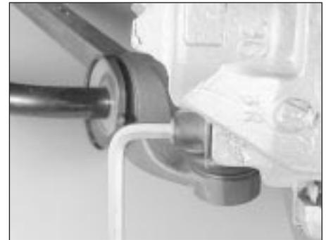
7.4 Undoing a caliper slide bolt
