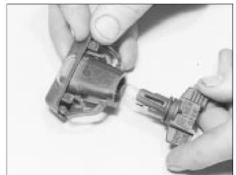
**3.30 Separate the unit to gain access to the number plate light bulb**
