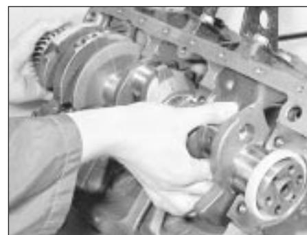
31.6 Placing the crankshaft in position
