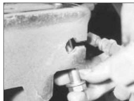
5.38 Removing a suspension crossmember securing bolt
