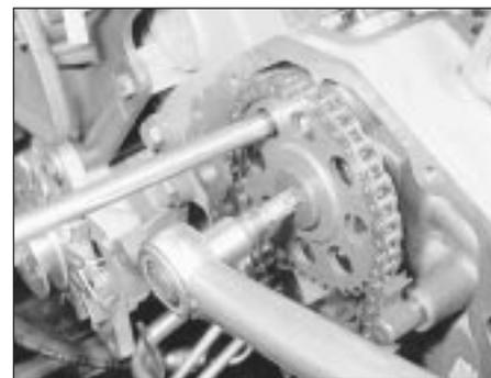
10.39 Slackening camshaft sprocket retaining bolt
