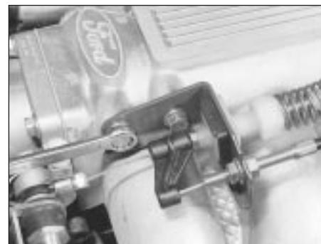
40.36 Unbolting the throttle cable bracket
