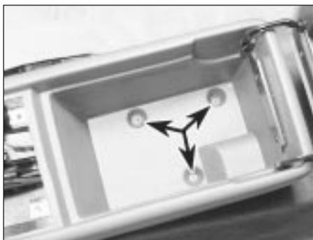
42.20a Centre console rear retaining screws (arrowed)
