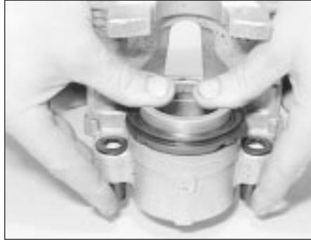
10.9 Pressing the piston into the bore
