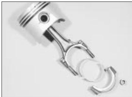
21.4 Piston, connecting rod, cap and bearing shells
