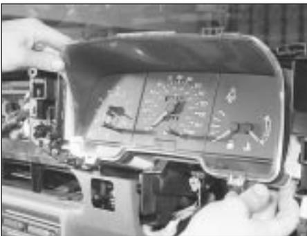
7.4b Removing the instrument cluster
