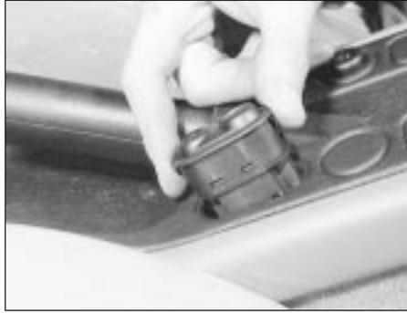
15.31 Removing a window operating switch
