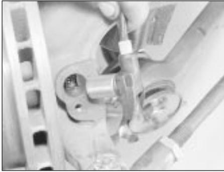
26.3 Removing a front sensor
