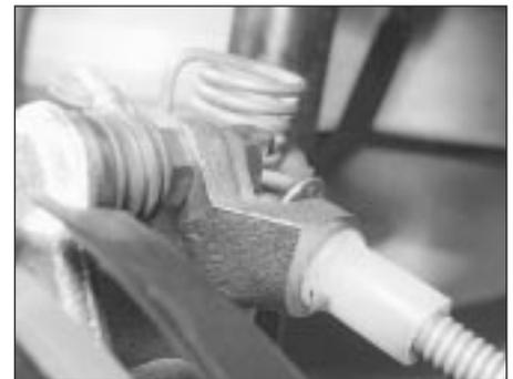
**23.4 Handbrake cable outer attached to caliper bracket**
