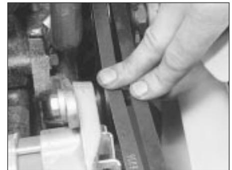
21.3 Checking drivebelt tension
