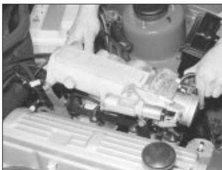
40.40a Removing the inlet manifold
