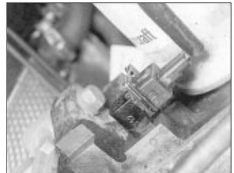
24.1 Crankshaft speed/position sensor (viewed from underneath)
