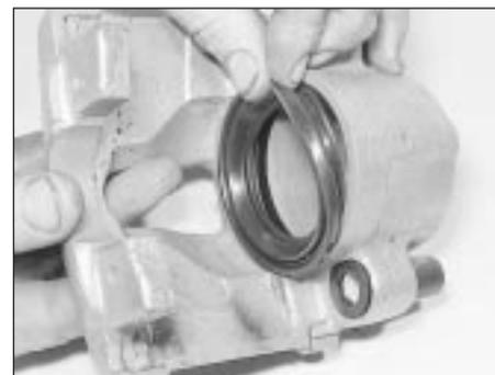
10.4 Removing the dust boot from a front caliper
