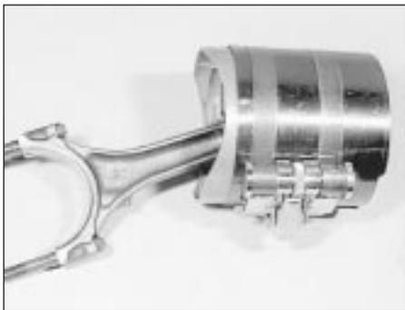
33.6a Piston with ring compressor fitted
