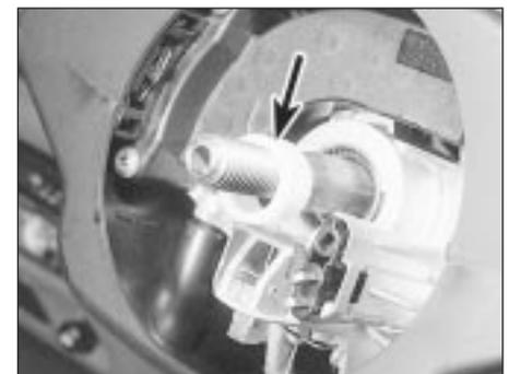
5.6 Spacer ring (arrowed) fits below steering wheel
