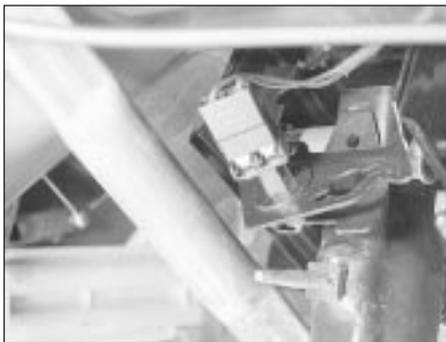
15.43 Stop-light switch fitted to brake pedal bracket
