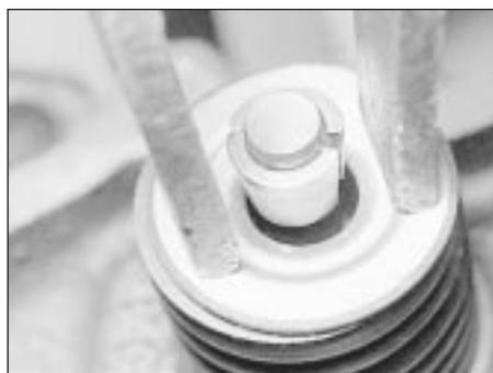
23.2a Compressing a valve spring to expose the collets
