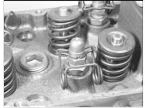
42.3 Cam follower ball-pins and spring clips fitted
