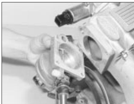
40.42b Removing the throttle body housing
