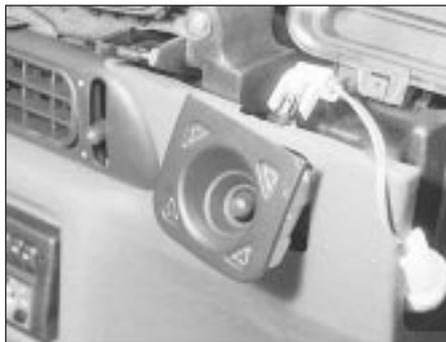
33.3 Removing the joystick fader
