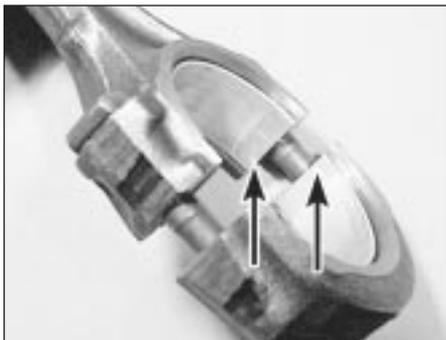
37.2 Big-end bearing shell lugs (arrowed) are adjacent
