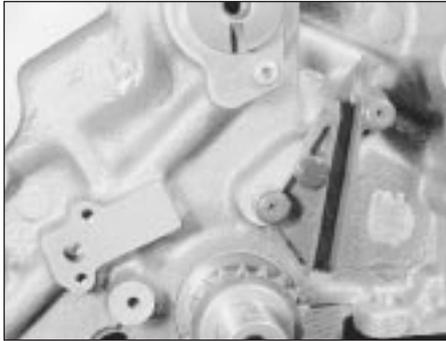
**36.15 Crankshaft and camshaft key and slot alignment**
