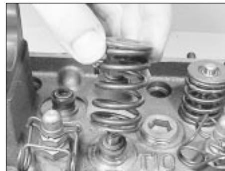
12.2b Removing a valve spring and cap
