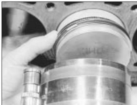
37.4a Fitting a piston ring compressor
