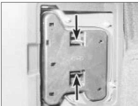
**3.27 Rear light cluster bulbholder retaining lugs (arrowed)**
