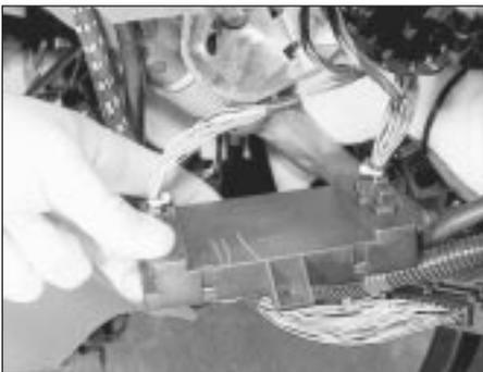
27.27 Removing the auxiliary warning system control module
