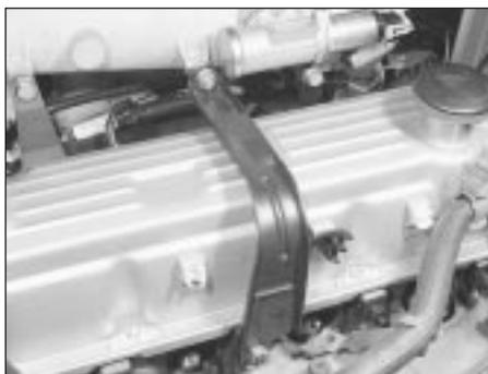
40.34 Inlet manifold-to-cylinder head bracing strut
