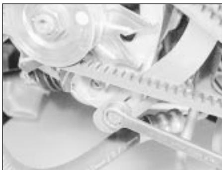
36.39a Alternator drivebelt tensioner strap bolt
