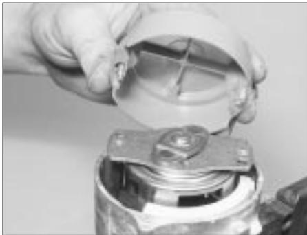
**39.9 Removing a rotor arm**
