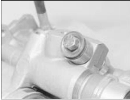
18.5 Hydraulic unit pump mounting bolt
