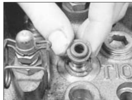
12.4 Removing a valve stem oil seal
