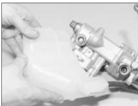
16.6 Removing the hydraulic fluid reservoir
