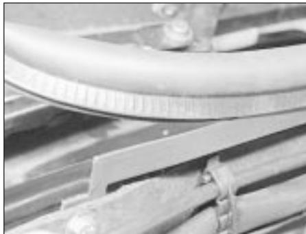
29.2 Pulling off the rubber sealing strip
