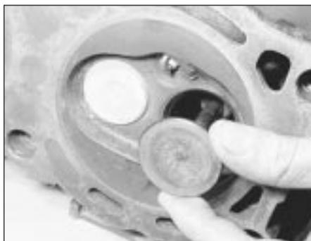
23.2c Removing an inlet valve
