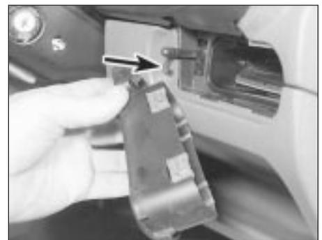
41.5 Remove the grille for access to the screw (arrowed)
