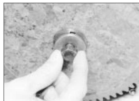
36.5 Camshaft gear washer and bolt
