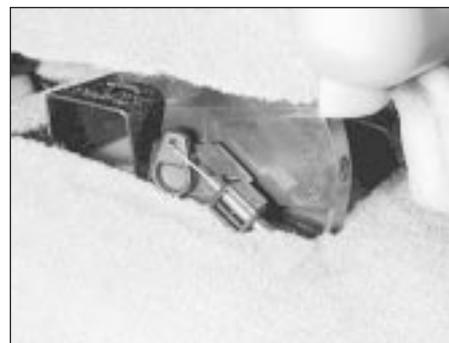
18.14 Rear heater control cable at nozzle
