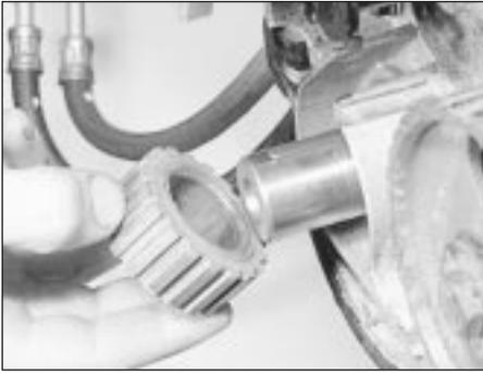
13.9 Removing the crankshaft sprocket
