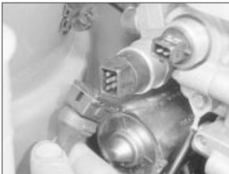
15.3d Disconnecting the pressure switch multi-plug
