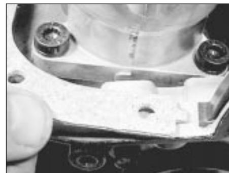
39.2 Locate the gasket tabs beneath the sealing strips
