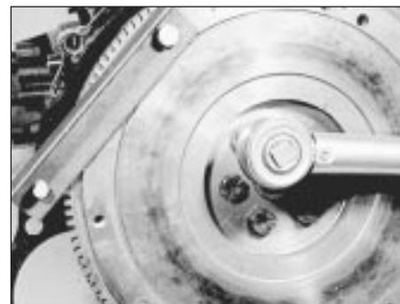
40.4b Tightening a flywheel bolt
