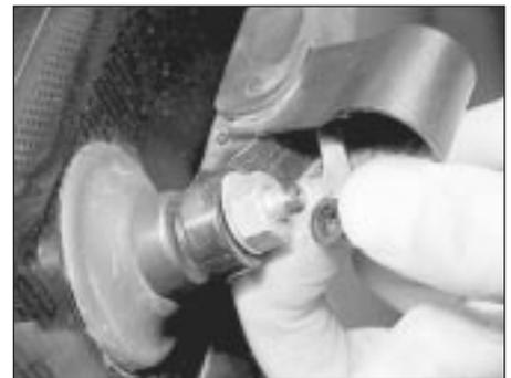
22.7 Disconnecting the rear wiper arm washer hose
