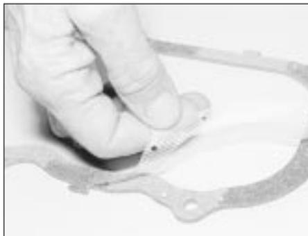
38.21 Peeling off rocker cover gasket protective shield
