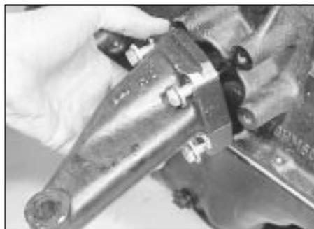
9.1b Removing an engine bearer arm
