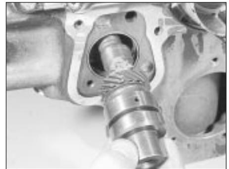
14.5b Removing the auxiliary shaft
