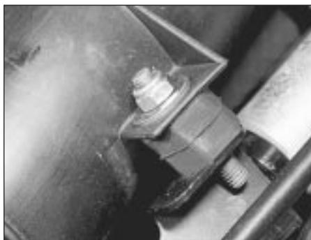
**38.17 Air intake tube retaining nut (fuel-injection DOHC)**
