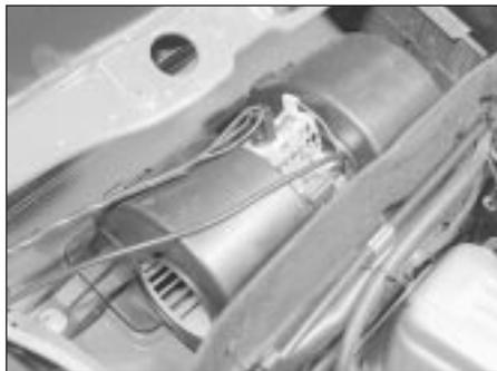
29.5 Blower motor showing wiring connections
