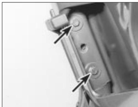
9.3 Boot lid retaining bolts (arrowed) - Saloon models
