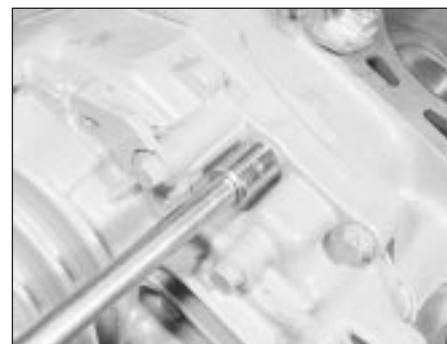
10.36 Removing a timing cover retaining bolt
