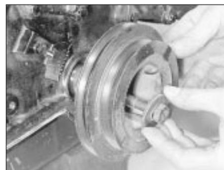
36.9 Fitting the crankshaft pulley
