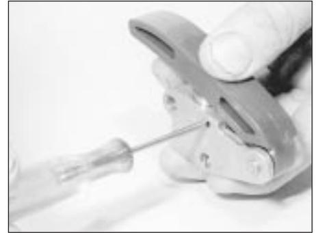
**36.20 Releasing timing chain tensioner pawl**
