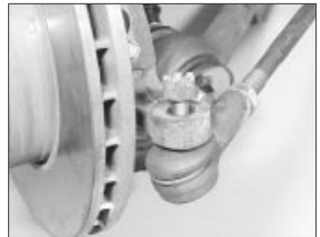
13.3 Track rod end balljoint nut unscrewed
