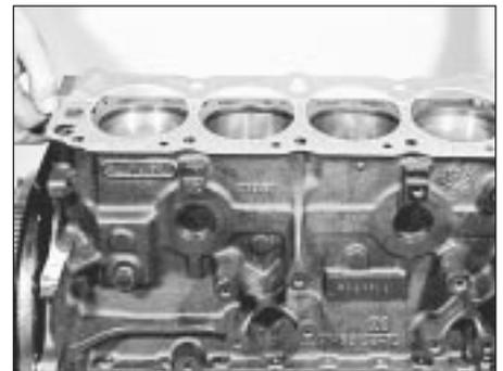
44.3 Fitting a new cylinder head gasket
