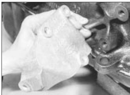
9.1c Removing the alternator bracket
