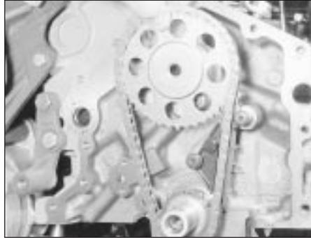
**36.18 Fitting timing chain and sprockets**
