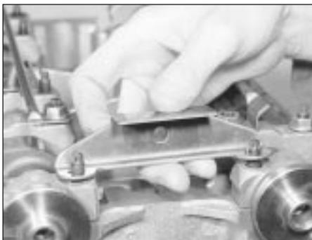
18.30c Fitting the timing chain guide plate
