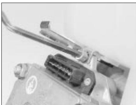
16.4 Undoing the reservoir securing screw
